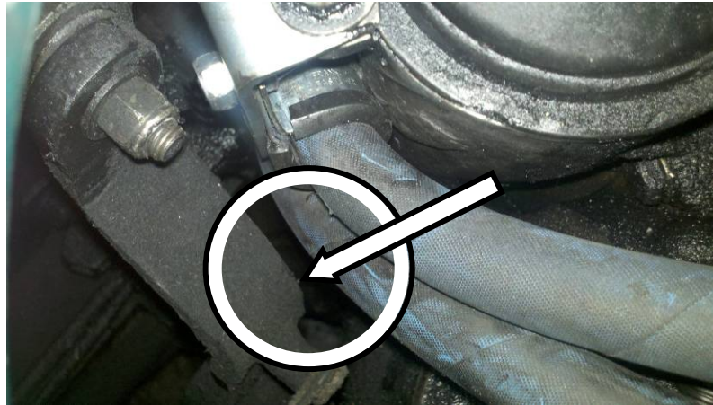
Figure 12 Clutch Arm to Fuel Line Clearance
