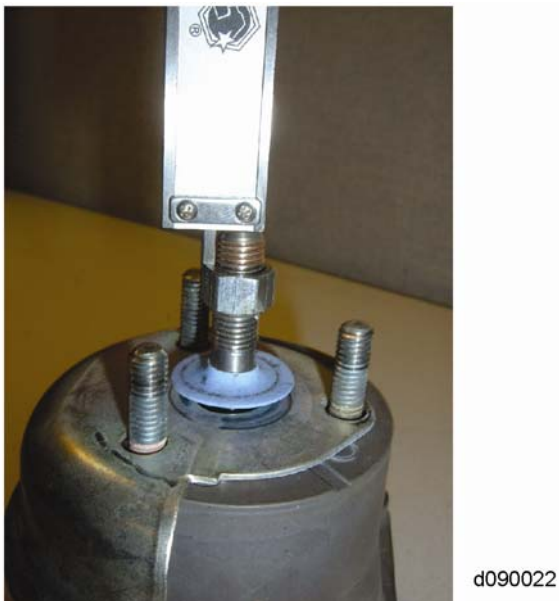
Figure 4 Installing Lower Lock Nut
