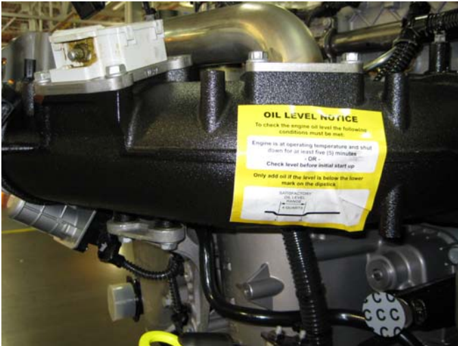
Figure 13 Installation of Oil Level Label
