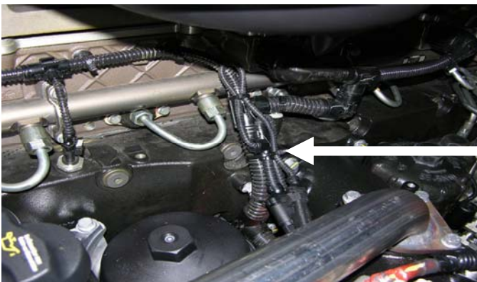
Figure 10 Installation of Adaptor Harness Using Tie Straps
