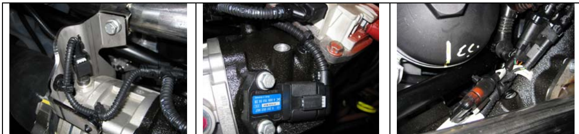
Figure 12 Installation of Adaptor Harness Clips
